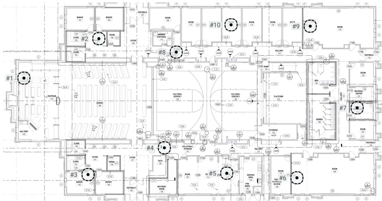
**Access Points on G300-MH-11 2024 1****Simulated Access Points on G300-MH-11 2024 1**
